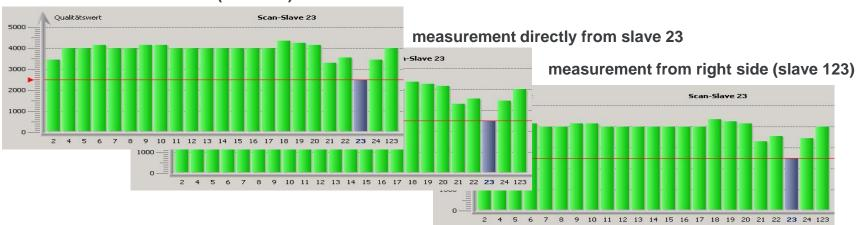
Case 5: Bus-termination is not powered correctly
